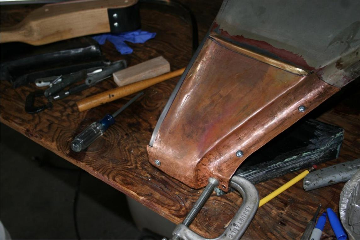
To form the needed piece I tried a brass plate, but could not get it to bend enough to fit the fender. I could not anneal the plate and make it soft enough to work. I anneal a copper plate and it worked out very well. By using a slapper and the English wheel I was able to make the part. Next I had to modify the brass trim part that was on top of this plate. All holes were drilled and the parts installed on the fender.
