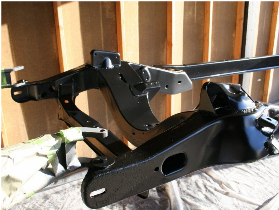
Frame after blasting and on rotator mounts for work and painting
