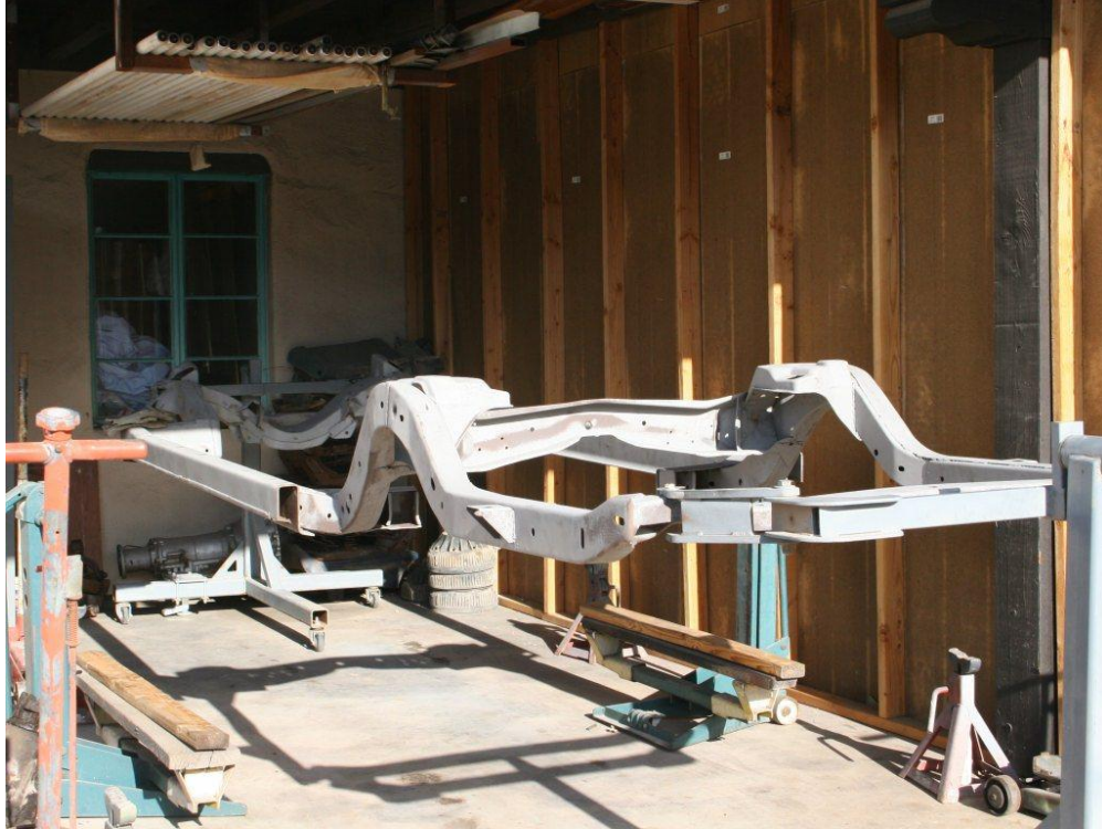
Frame after blasting and on rotator mounts for work and painting
